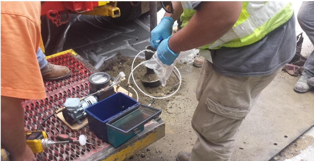
Figure 3 - A sample in a Tedlar bag is retrieved and ready to take a reading from using a PID meter (lower left).
