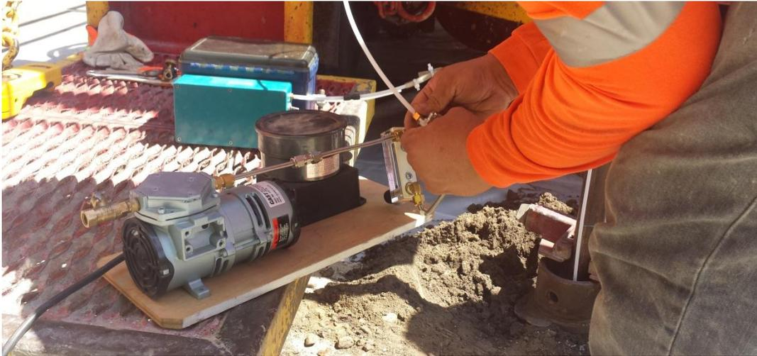
Figure 2 - Connecting the vacuum pump to the air-line of the Simulprobe.
